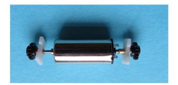
Railcar / DMU 101 Poole manufactured armatures Ref GF8169 has been replaced with CM2020-3 comes with bearings and correct gears inc. wires attaced for power supply.
